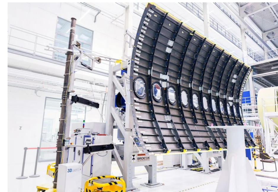
3D.aero's SurfEyes measuring the panels back interface edge.
