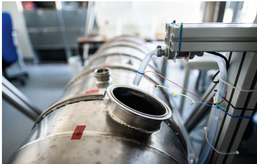
Airbus XR fill level gauging demonstration tank.
