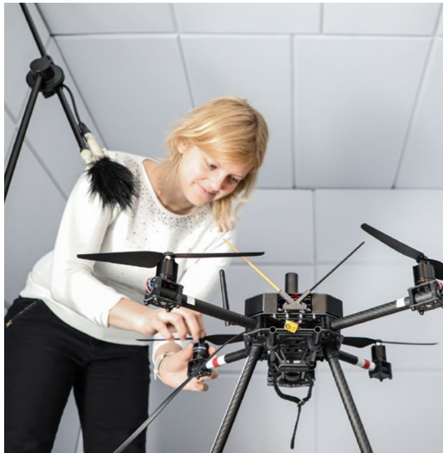
A drone is prepared for audio recording in the anechoic chamber at the ZAL.
